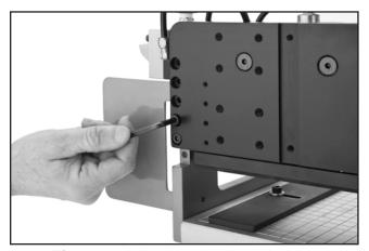
Figure 9. Adjusting the clamp height.
